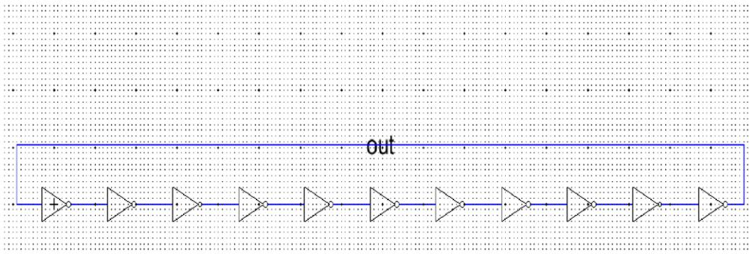
Fig.2 Schematic of 11 stage Ring Oscillator
