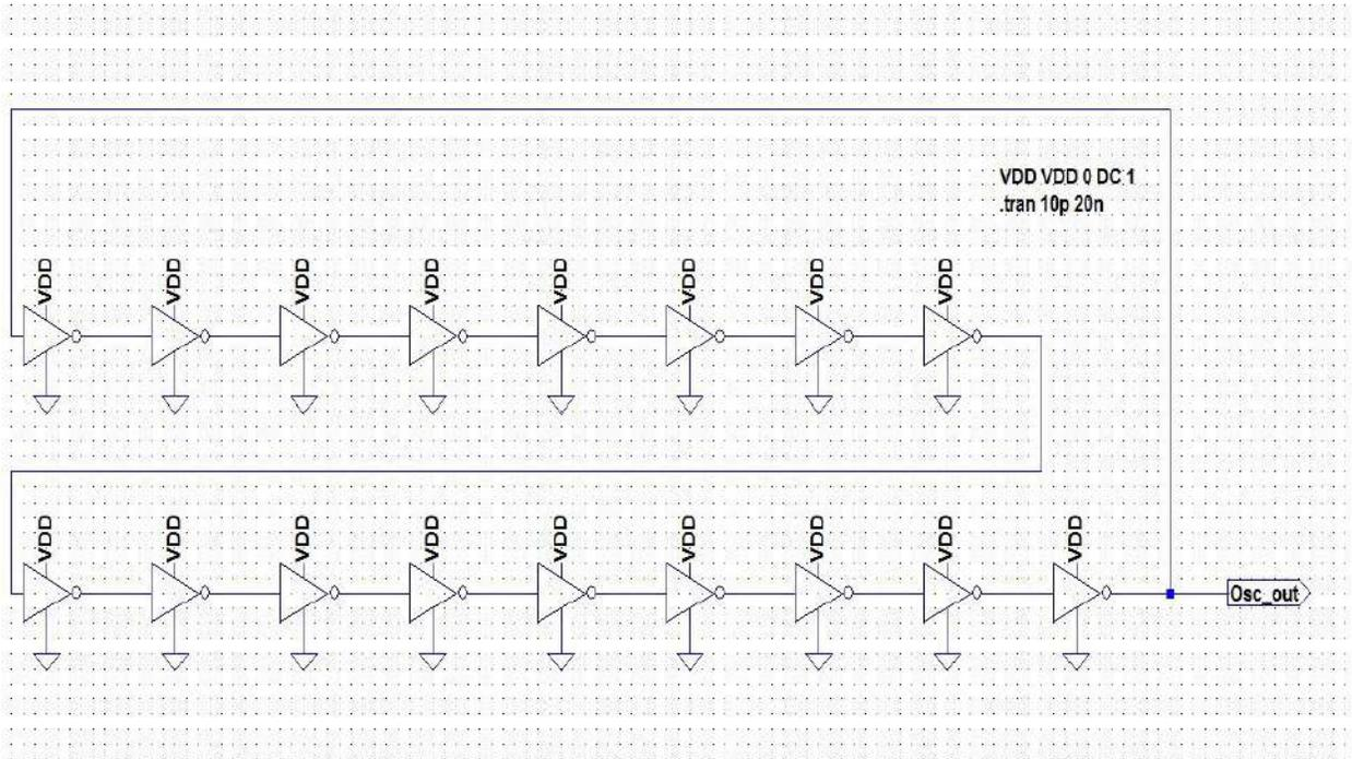
Figure 23: Schematic for Ring Oscillator
