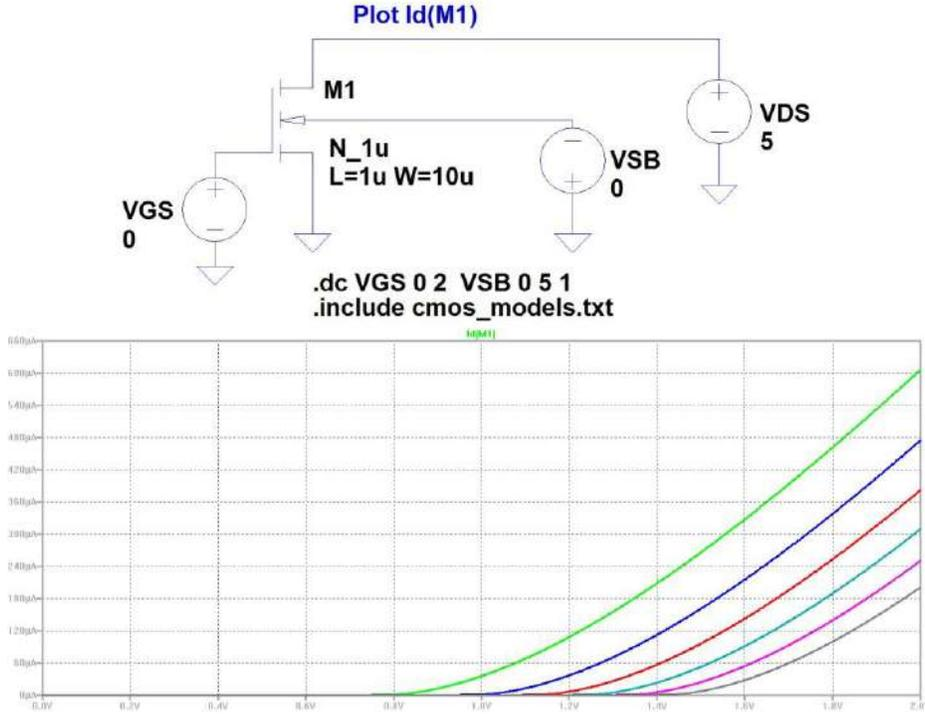
Figure 6: Schematic and plot for Id characteristics for NMOS 1u model
