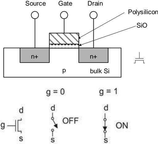
Figure 2 : NMOS structure, symbol and logic
