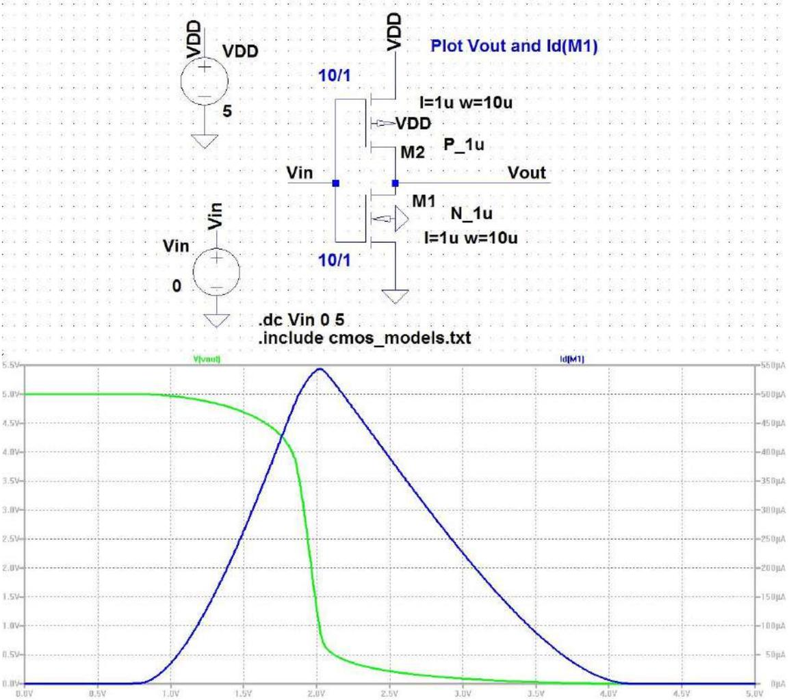
Figure 5: Voltage Current characteristics for a long channel inverter
