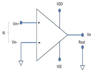
Fig. 3 Showing input and Output Resistance
