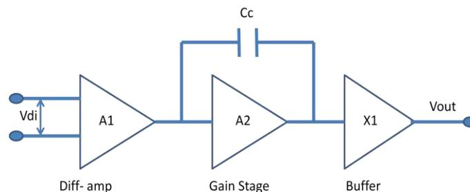
Fig 1.1 Block Diagram of 2 stage Operational Amplifier with output buffer.
