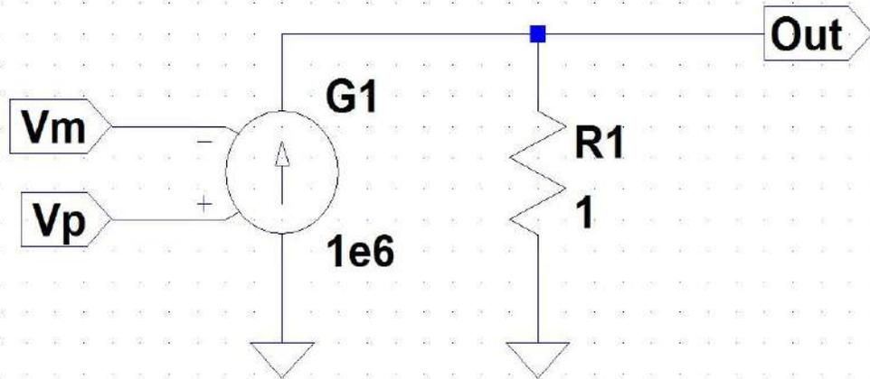
Figure 3: Ideal Operational Amplifier using VCCS
