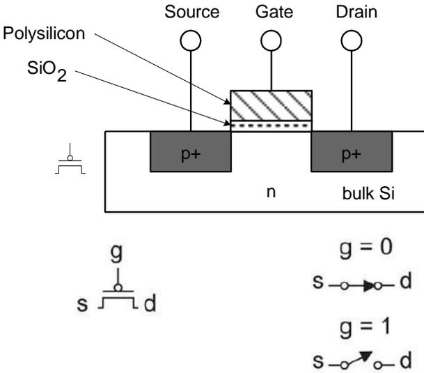
Figure 3: PMOS structure, symbol and logic
