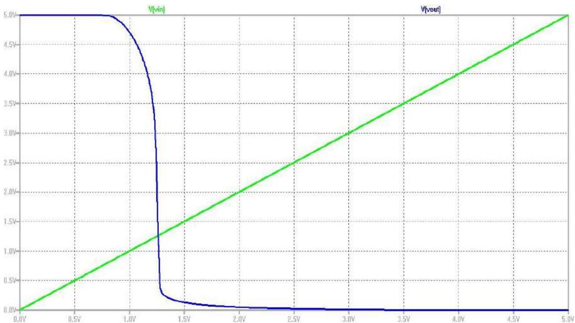
Figure 29: DC analysis plot for 3 input NAND Gate
