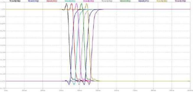
Fig.12 Simulation plot for 51 stage Ring Oscillator
