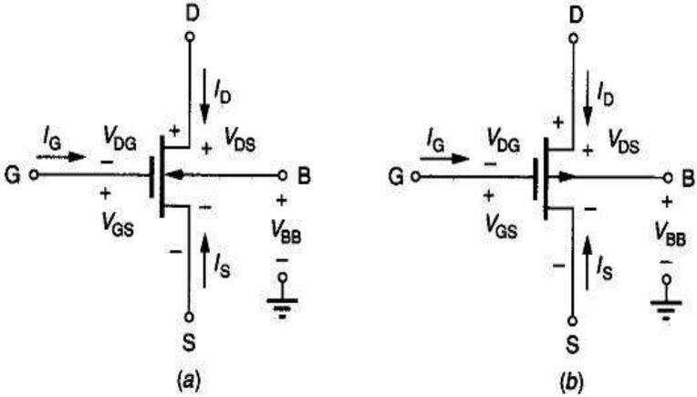
Figure 2: Basic voltage and current notations for MOSFET
