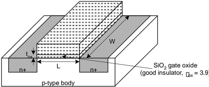
Figure 1: Basic MOS Transistor
