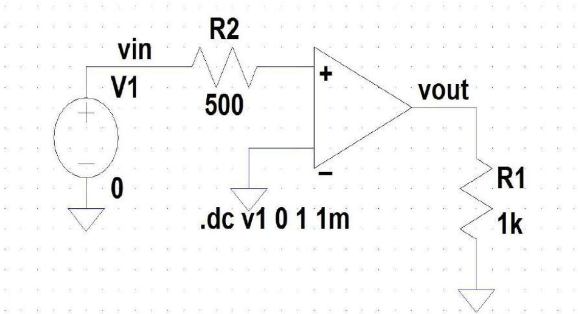
Figure 7: Ideal Opamp in non-inverting configuration
