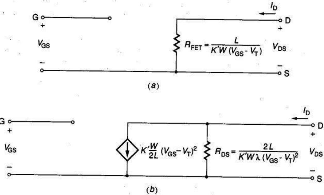
Figure 3 Equivalent Circuits of MOSFET in Ohmic Region and Saturation regions respectively
