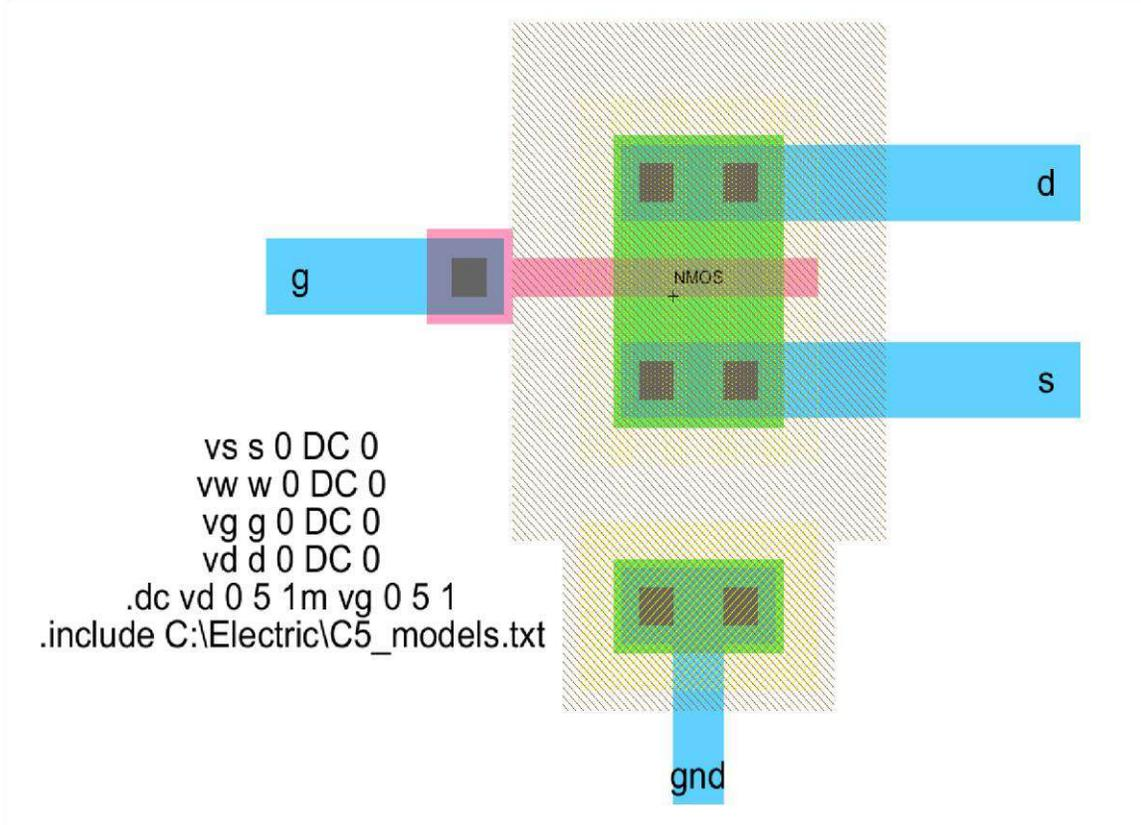
Figure 17: Layout and spice code for DC characteristics for NMOS
