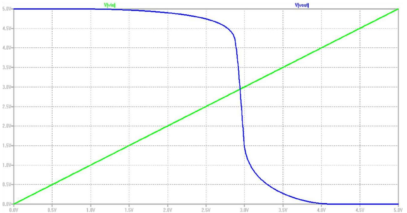
Figure 25: DC Analysis plot for 3 input NAND Gate
