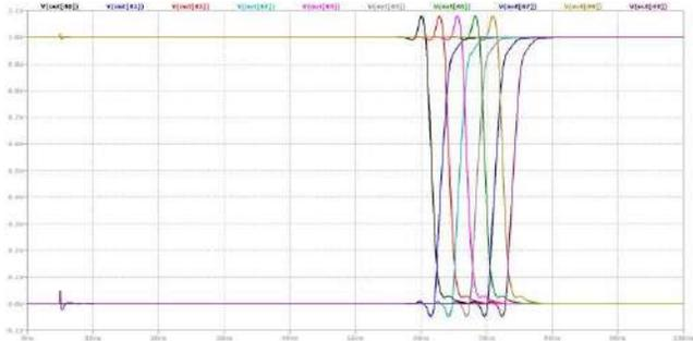
Fig.14 Simulation plot for 51 stage Ring Oscillator
