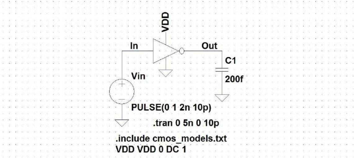
Figure 21: Schematic for Digital Inverter using variable load
