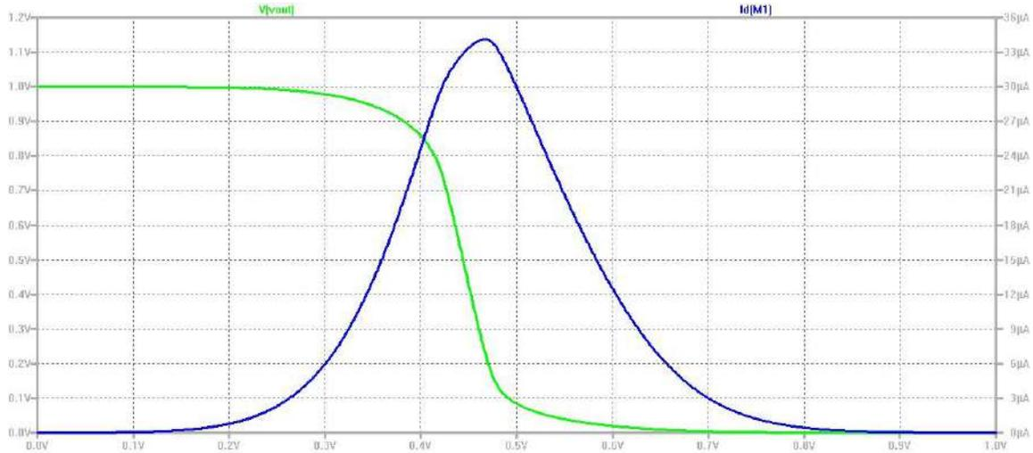
Figure 6: Voltage Current characteristics for a short channel inverter
