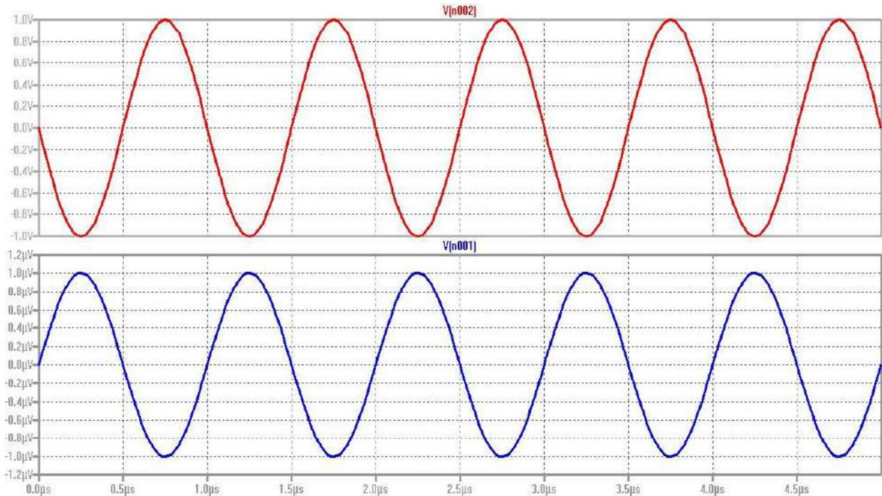
Figure 10: Plot for Ideal Opamp in inverting configuration
