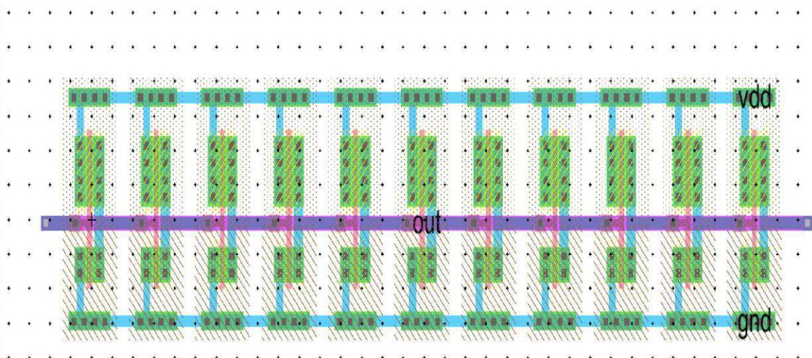
Fig.3 Layout of 11 stage Ring Oscillator
