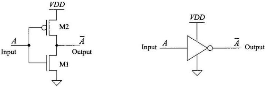
Figure 3: CMOS Inverter, schematic and logic symbol
