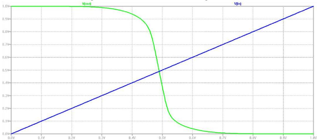
Figure 20: DC Simulation plot for CMOS Inverter
