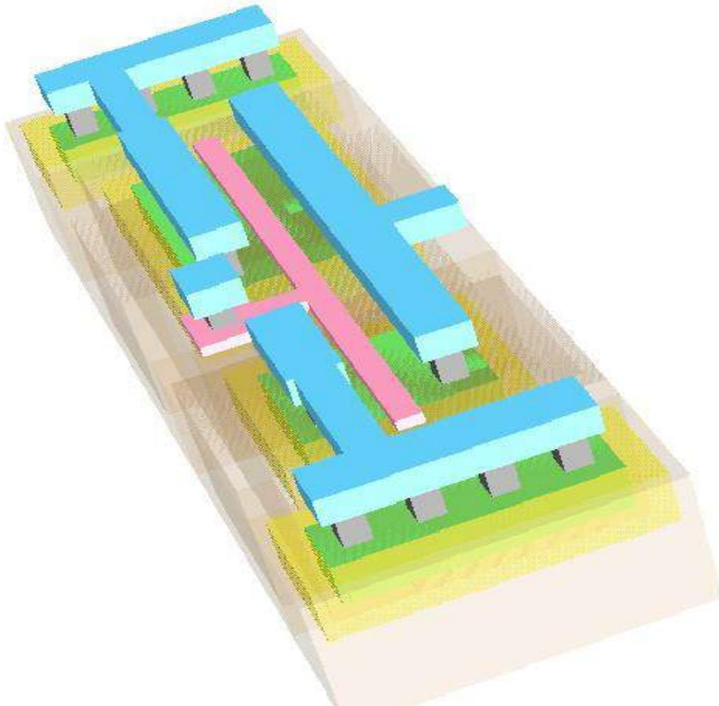
Figure 13: 3D View of a CMOS Inverter
