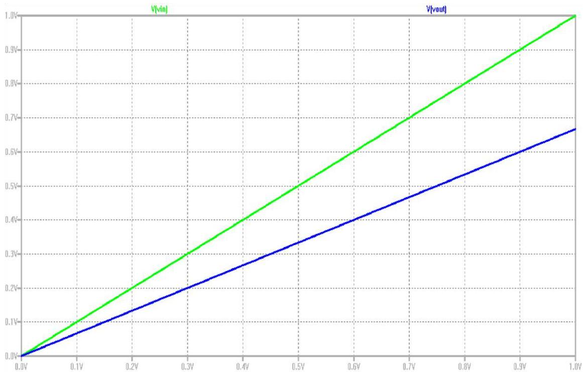
Fig 4: Resistance divider schematic and dc sweep analysis plot
