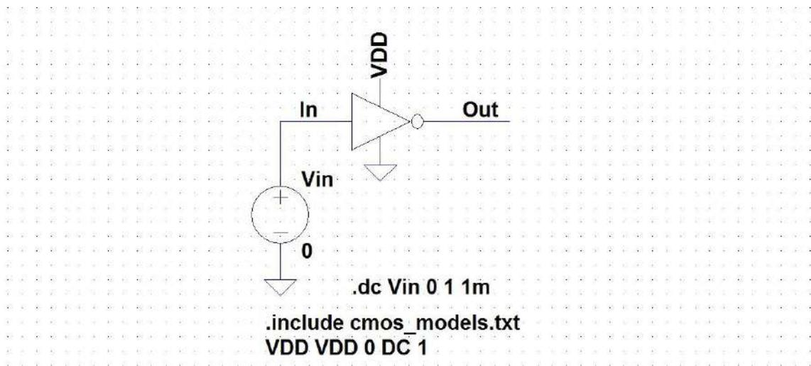
Figure 19: DC Simulation for Digital Inverter
