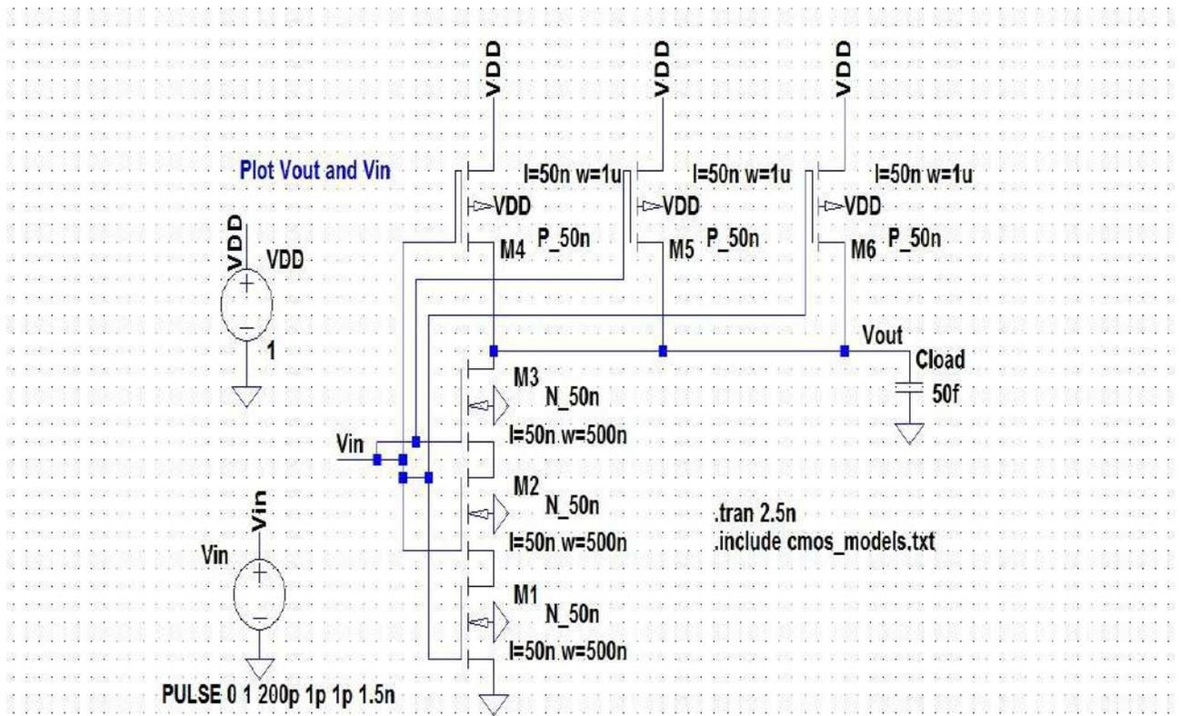
Figure 30: Schematic for 3 input NOR Gate
