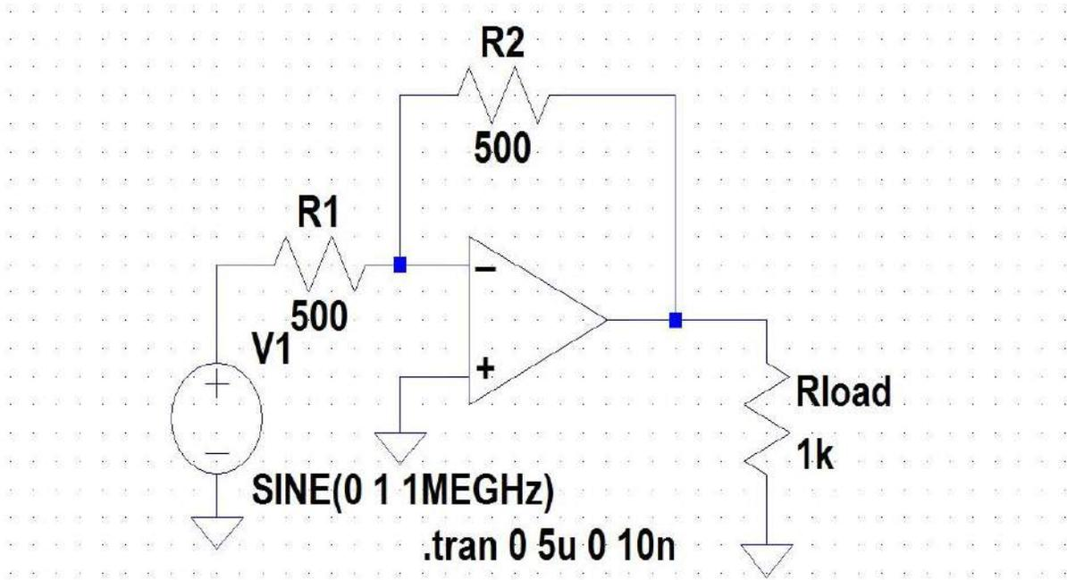
Figure 9: Schematic for Ideal Opamp in inverting configuration
