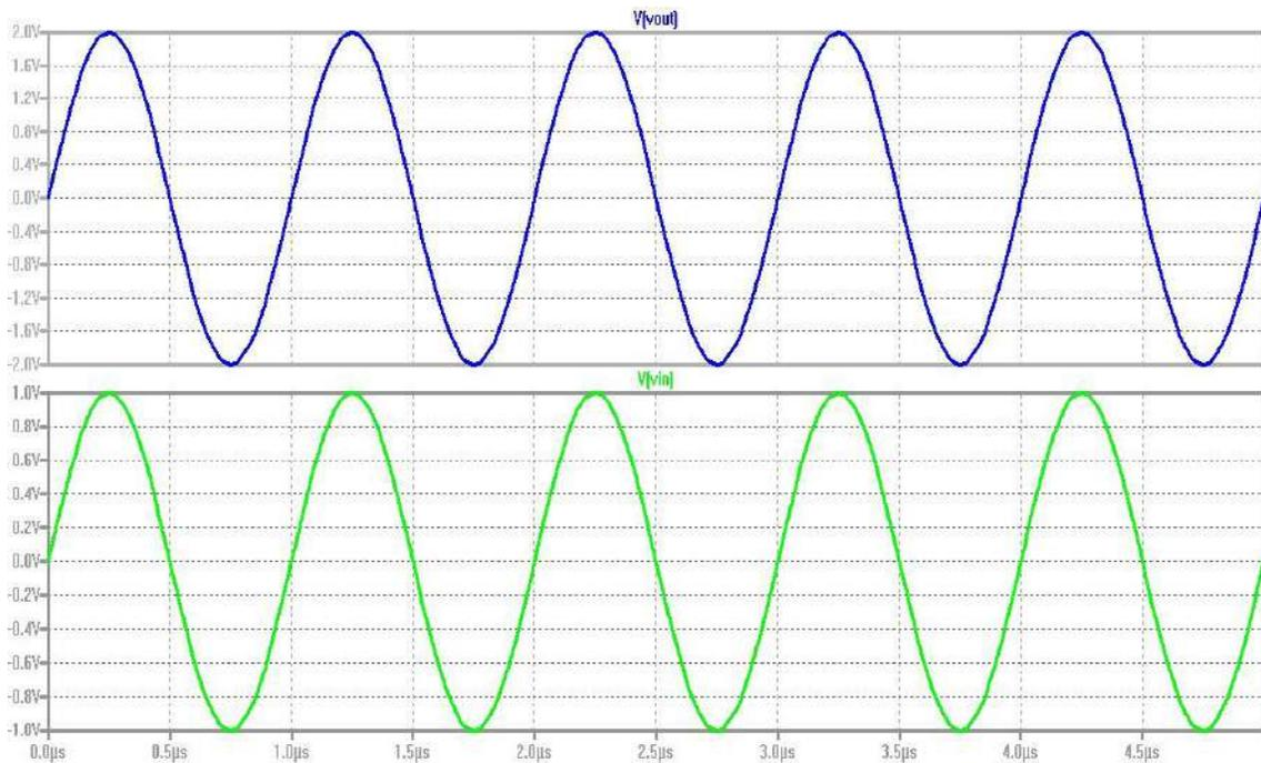
Figure 12: Plot for Ideal Opamp in non-inverting configuration
