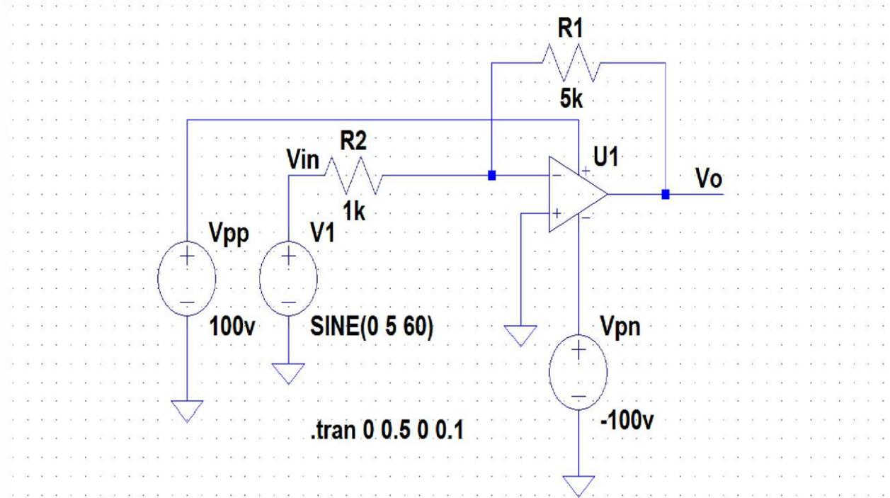
Figure 1: Schematic of Ideal Opamp simulation
