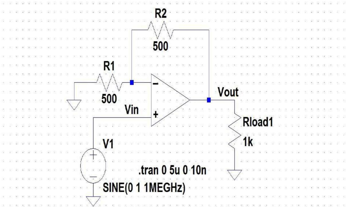
Figure 11: Schematic for Ideal Opamp in non-inverting configuration
