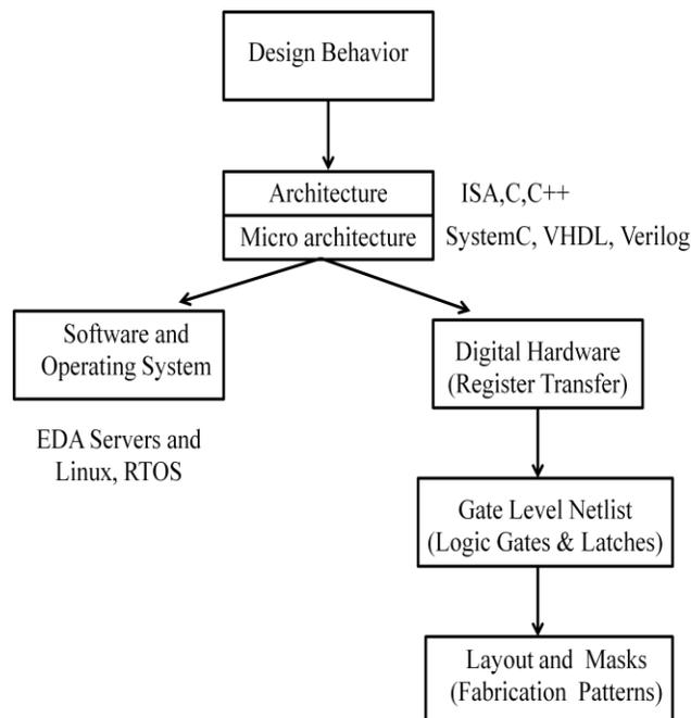
Fig 2 Design representation levels and formats associated
