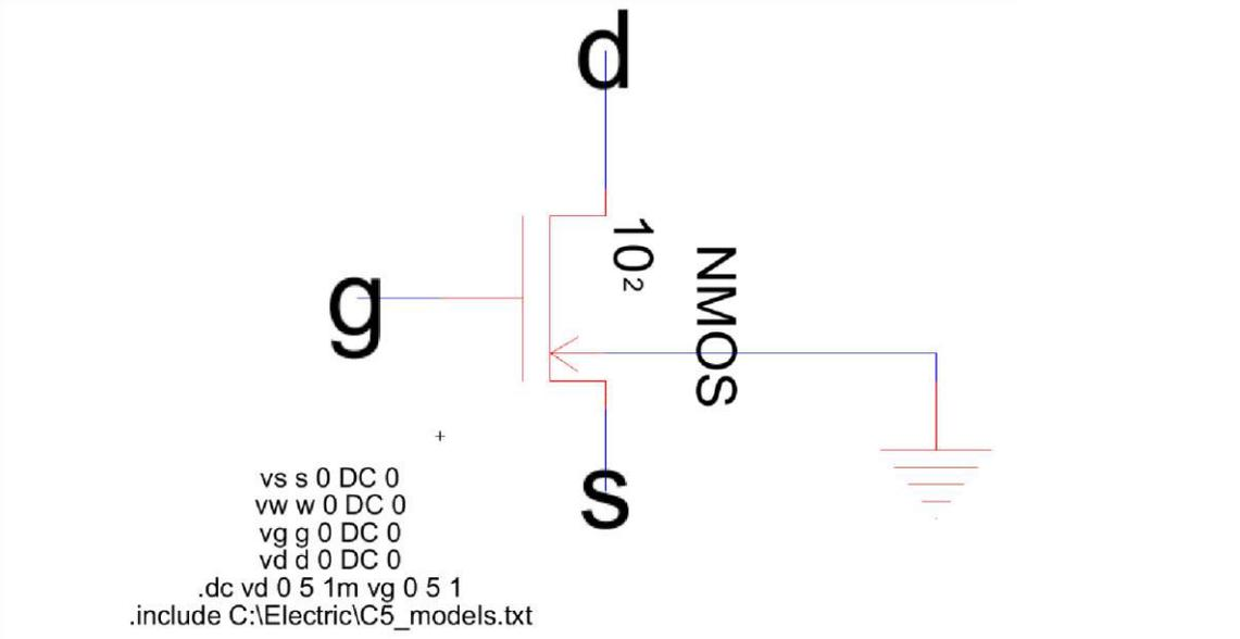
Figure 16: Schematic and spice code for DC characteristics for NMOS
