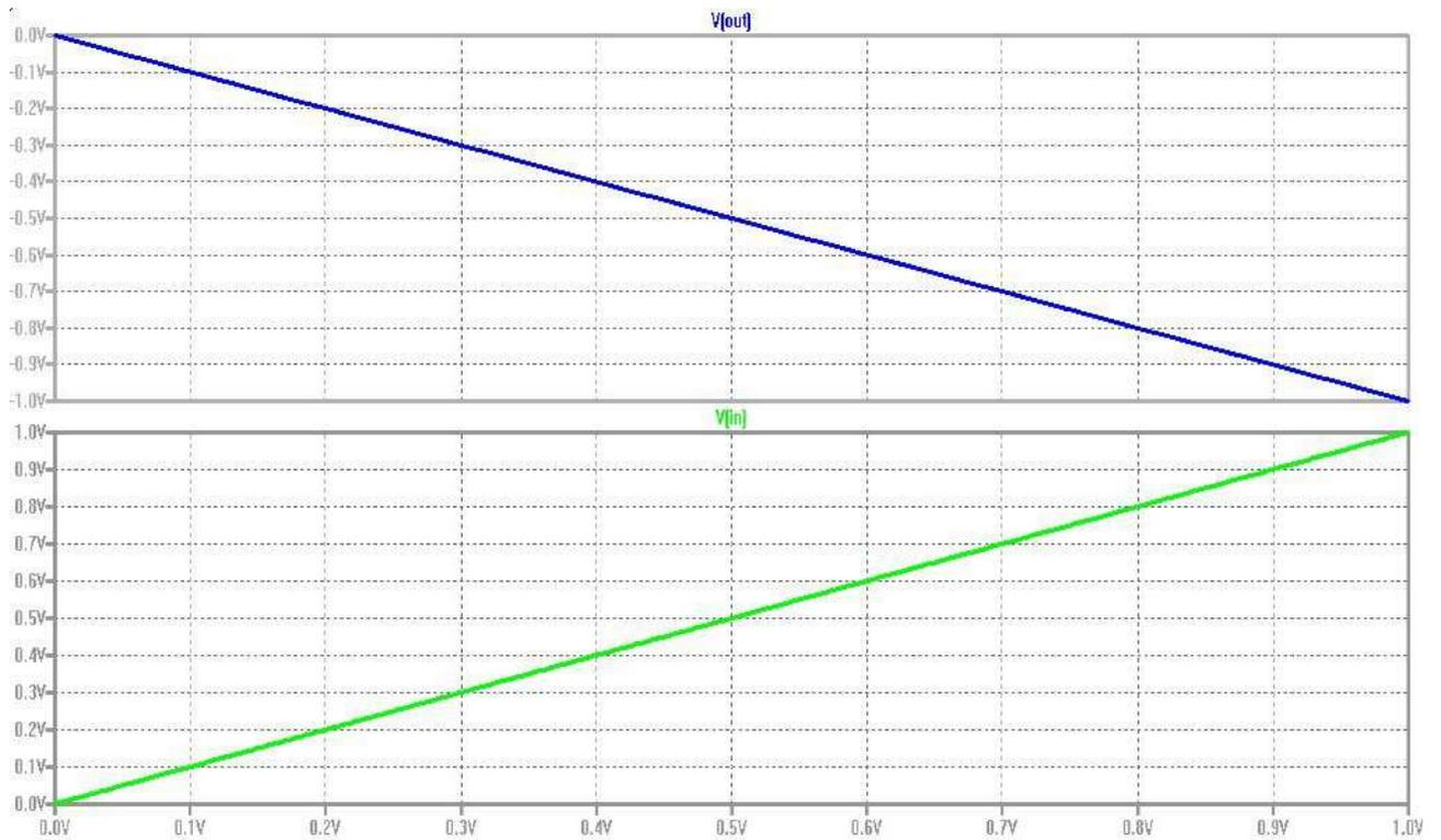
Figure 6: Plot for Ideal Opamp in inverting configuration
