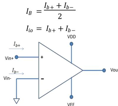
Fig.4 Op-amp input bias current and input offset current
