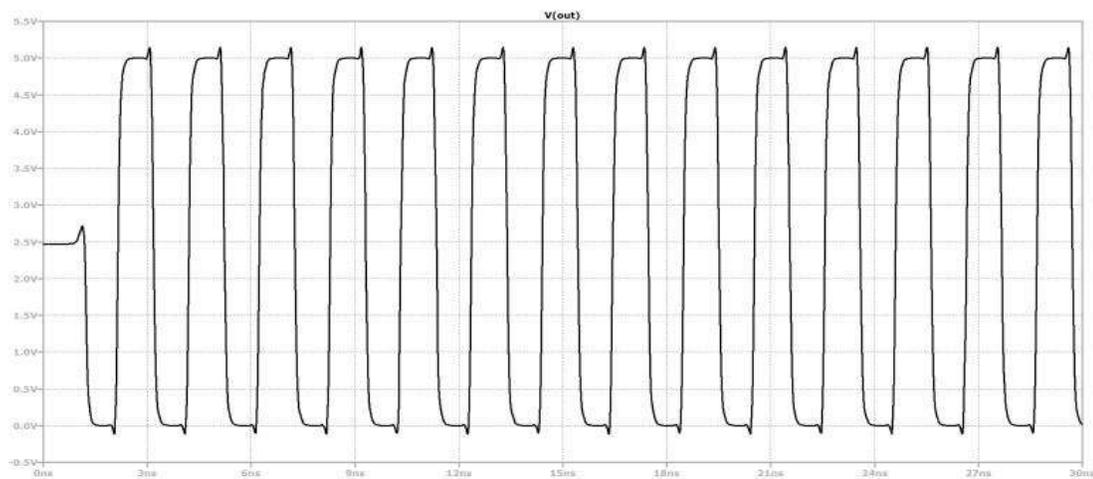
Fig.4 Transient plot for 11 stage Ring Oscillator
