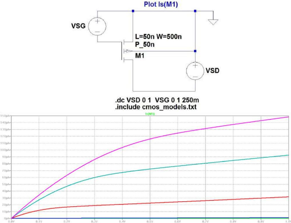
Figure 10: Schematic and plot for Is characteristics for PMOS 50n model
