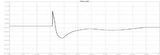
Fig.9 Simulation plot for 51 stage Ring Oscillator (Transient 100n)
