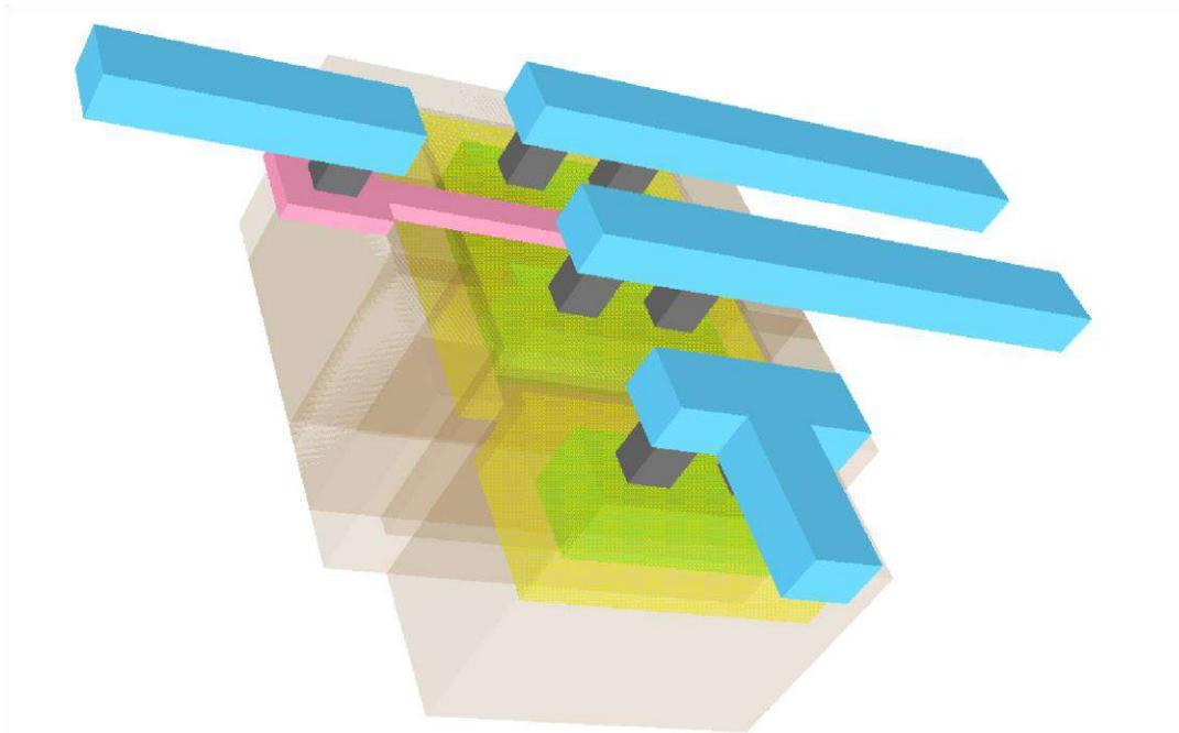
Figure 18: 3D view for NMOS Transistor
