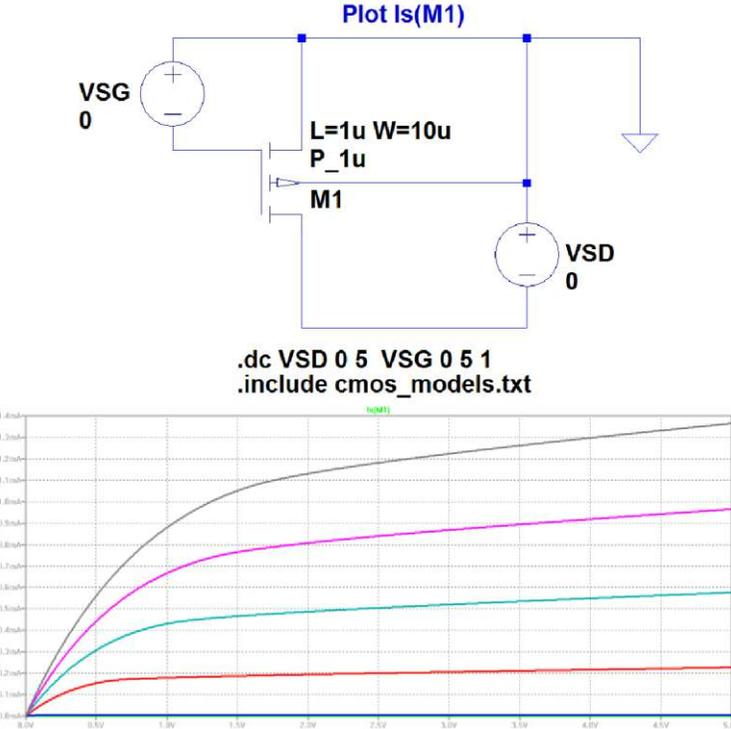
Figure 5: Schematic and plot for  $I_s$  characteristics for PMOS 1u model
