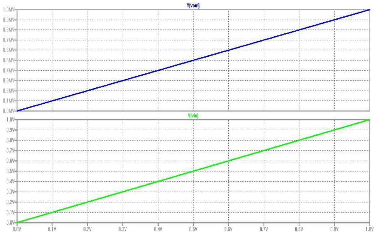
Figure 8: Plot for Ideal Opamp in non-inverting configuration
