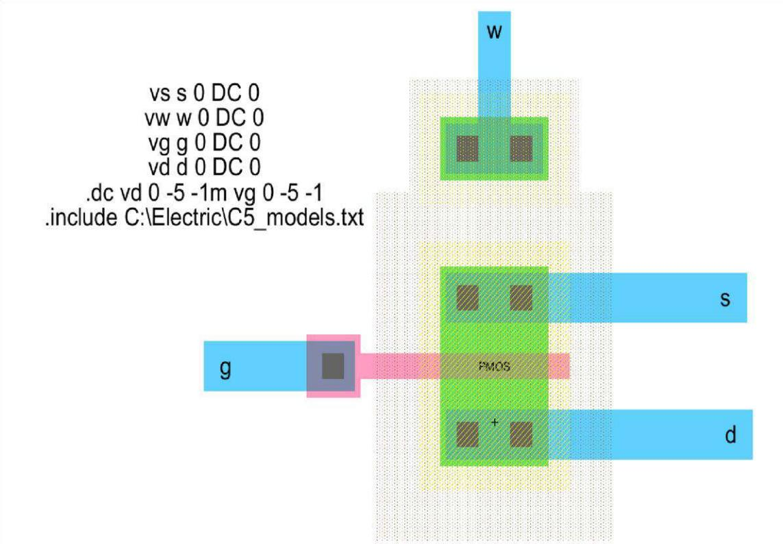
Figure 13: Layout and spice code for DC characteristics for PMOS
