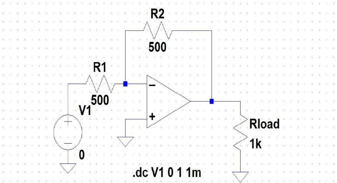
Figure 5: Ideal Opamp in inverting configuration
