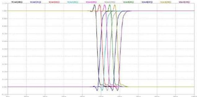
Fig.13 Simulation plot for 51 stage Ring Oscillator
