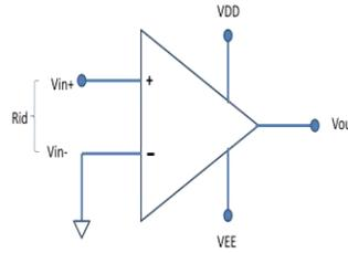
Fig. 2 Input Differential Resistance
