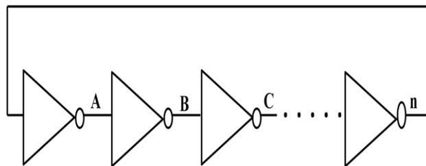
Fig.1 Ring Oscillator realization with n digital inverters
