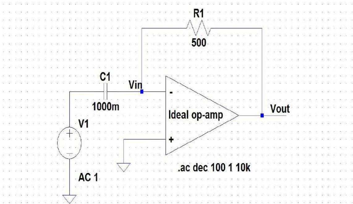
Figure 15: Schematic for Ideal Opamp used as a Differentiator
