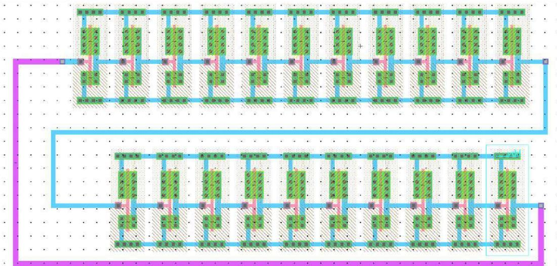
Fig.6 Layout of 21 stage Ring Oscillator
