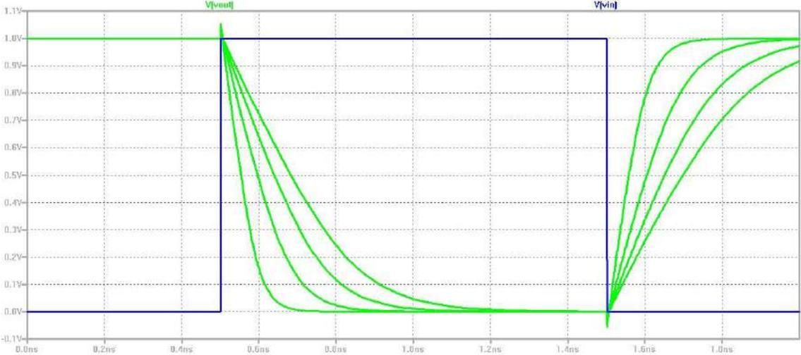
Figure 9: Voltage Transfer characteristics for CMOS inverter with varying load and pulsating input
