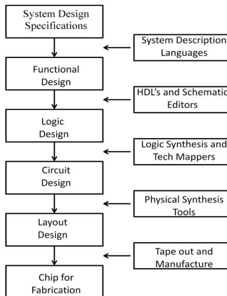
Fig. 3 Traditional VLSI Design Flow
