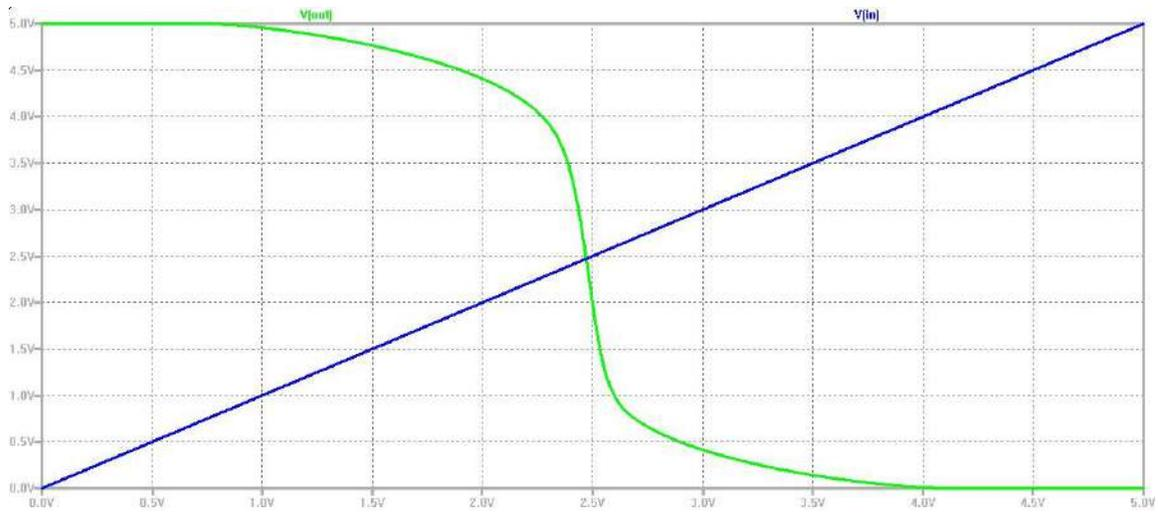
Figure 12: DC Characteristics for a CMOS Inverter
