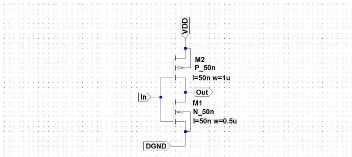
Figure 17: Schematic for Digital Inverter
