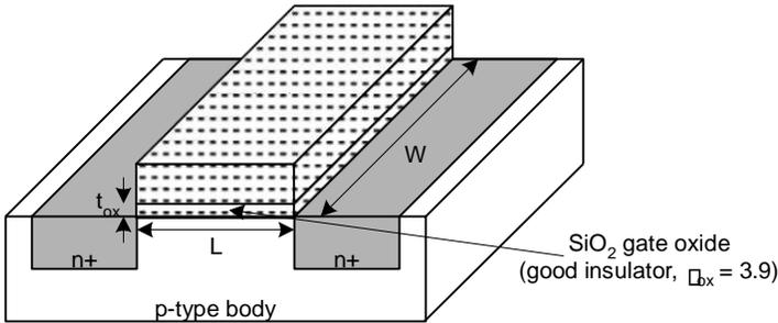
Figure 1: Basic MOS Transistor
