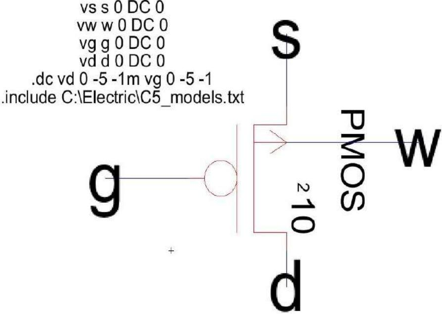
Figure 12: Schematic and spice code for DC characteristics for PMOS
