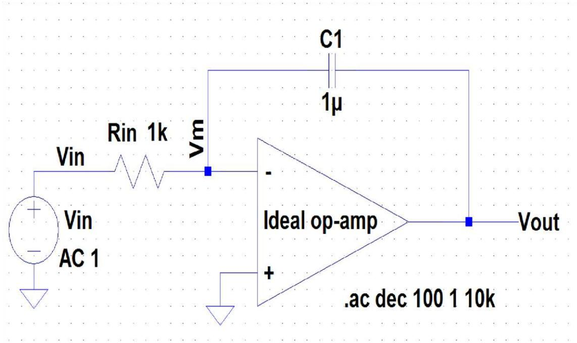
Figure 13: Schematic for Ideal Opamp used as a Integrator
