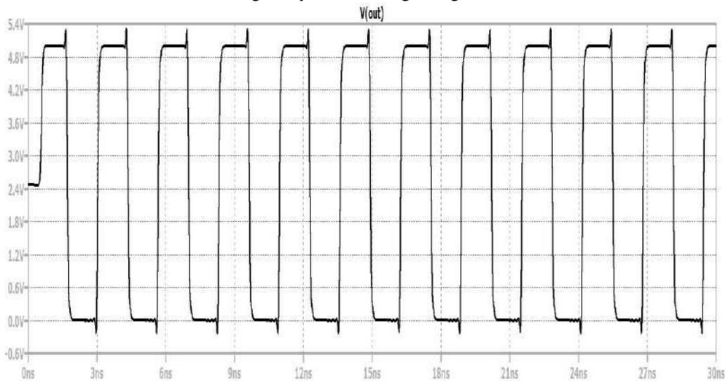
Fig.7 Simulation plot for 21 stage Ring Oscillator
