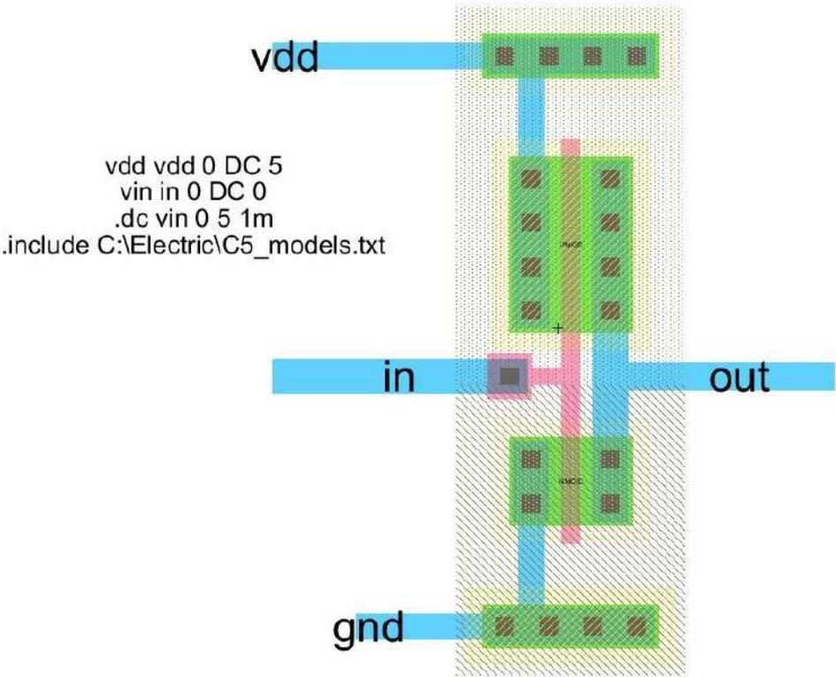
Figure 11: CMOS Inverter icon and layout with respective simulation SPICE scripts
