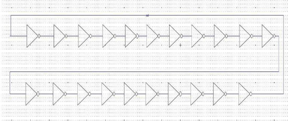
Fig.5 Schematic of 21 stage Ring Oscillator
