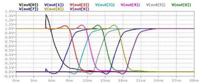
Fig.10 Simulation plot for 51 stage Ring Oscillator
