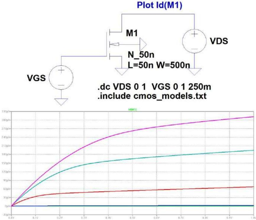
Figure 8: Schematic and plot for  $I_d$  characteristics for NMOS 50n model
