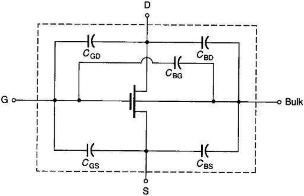
Figure 4: Capacitor lumped model
