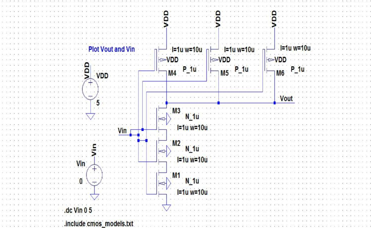
Figure 24: Schematic for 3 input NAND Gate
