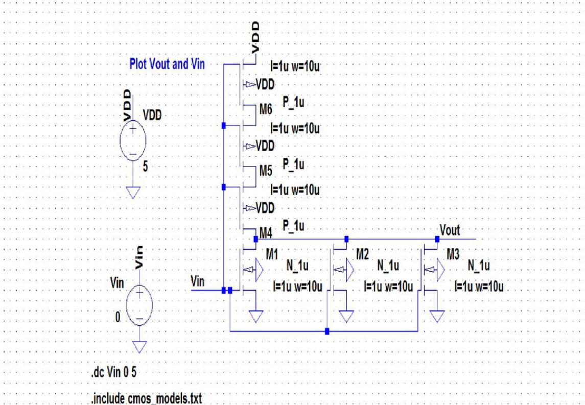
Figure 28: Schematic for 3 input NOR Gate
