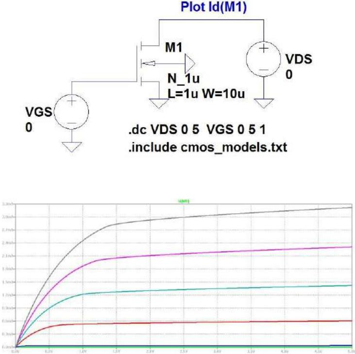
Figure 4: Schematic and plot for  $I_d$  characteristics for NMOS 1u model
