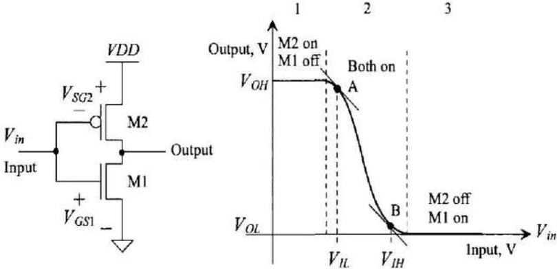
Figure 3: CMOS Inverter, DC transfer characteristics
