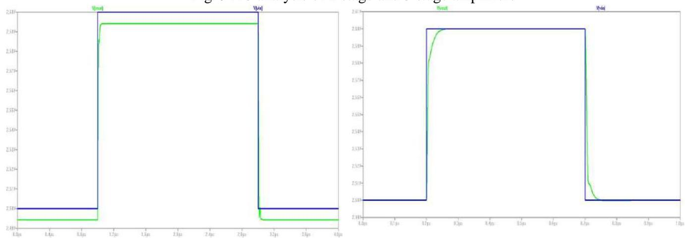
Fig.10 Transient analysis for 2 and 3 stage amplifiers
