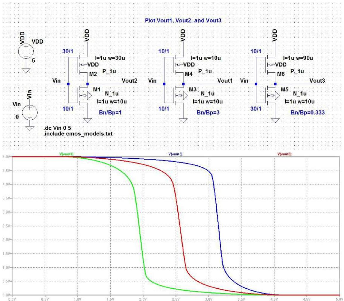
Figure 7: Voltage characteristics for different widths CMOS inverters
