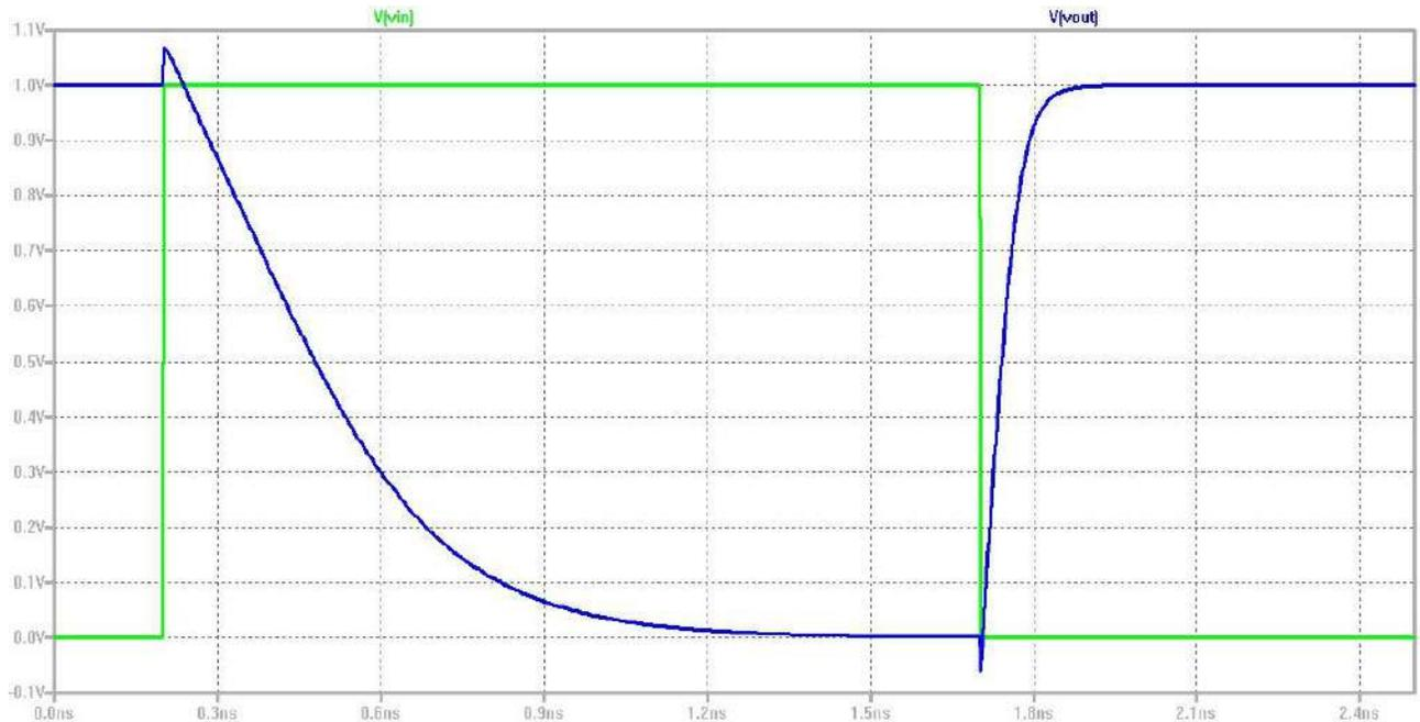
Figure 31: Transient plot for 3 input NOR Gate
