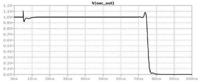
Fig.8 Simulation plot for 51 stage Ring Oscillator (Transient 30 n)
