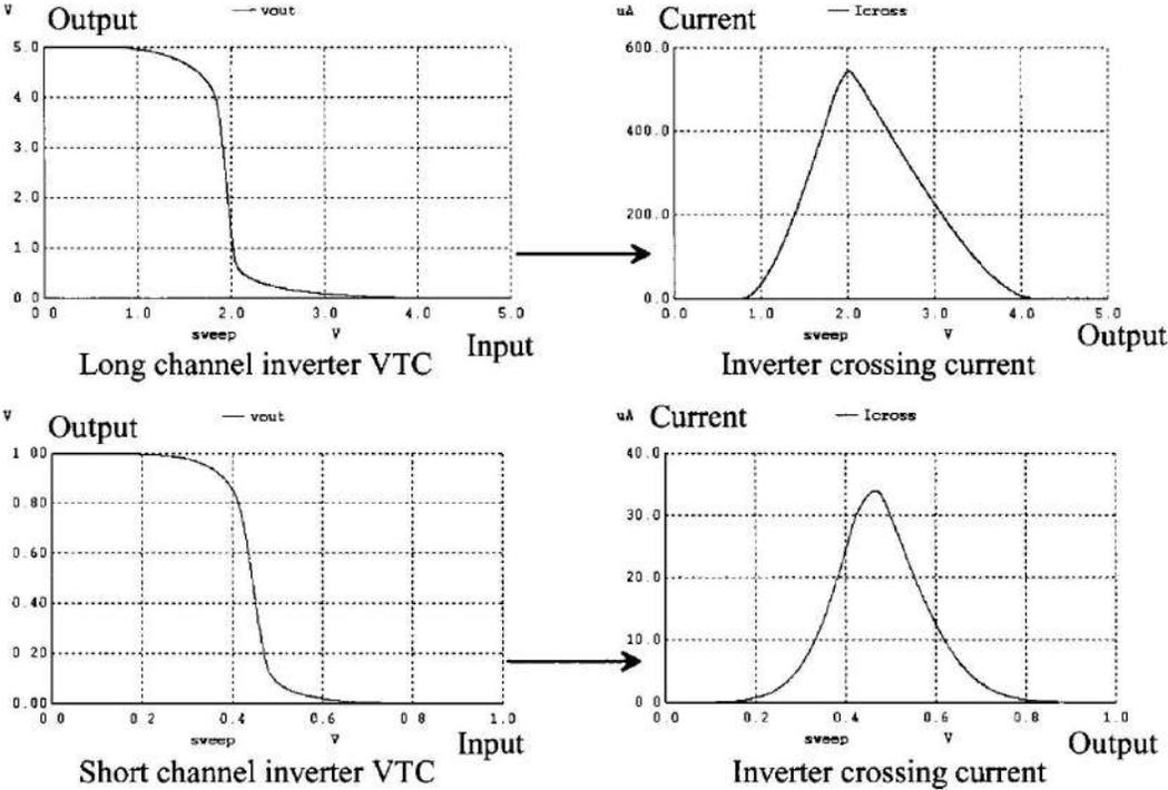
Figure 4: Voltage transfer curves (VTCs) for a long and a short channel inverter. In this lab simulations are performed using default and cmos\_models that includes 300nm c5 process, 1u model and 50n model.
