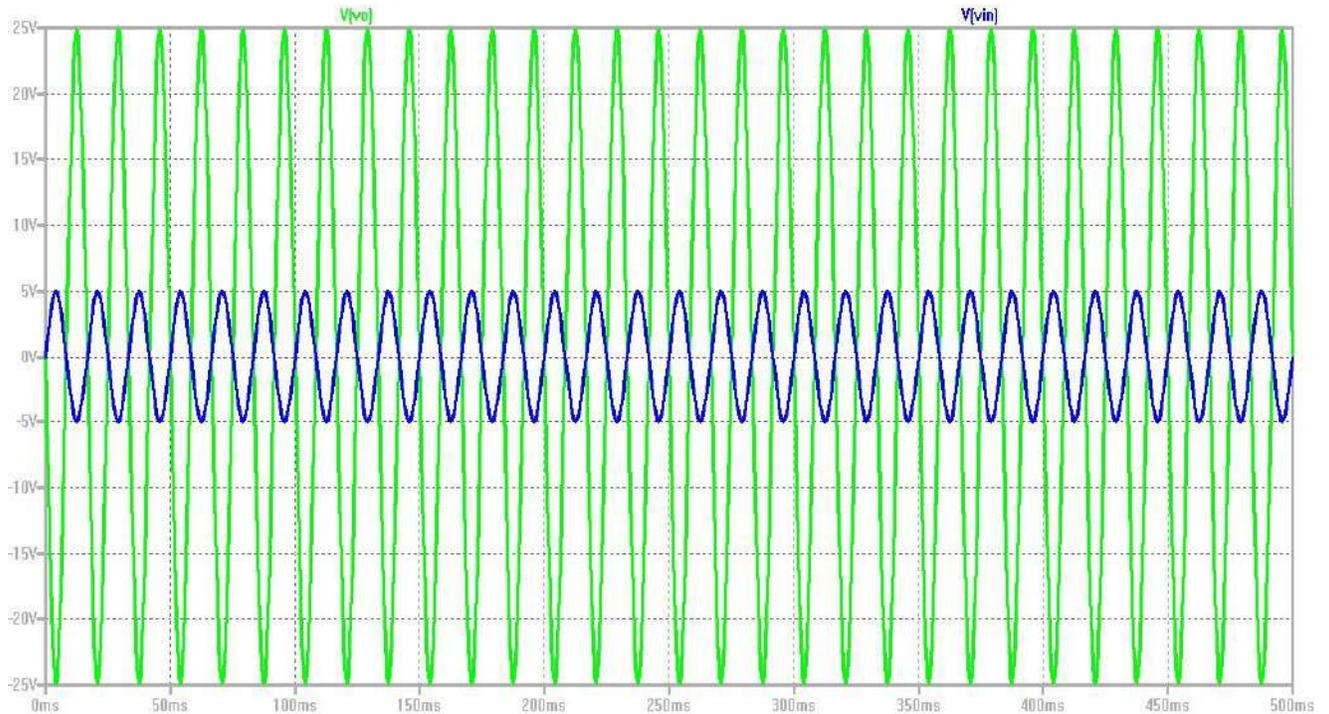
Figure 2: Plot for Vout vs Vin for Ideal Opamp Schematic in figure 1
