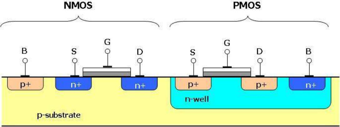
Figure 2 : Side view of CMOS Inverter
