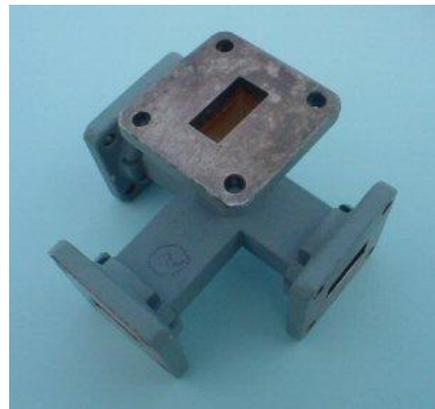
phase. A signal injected into the E-plane port will also be divided equally between ports 1 and 2, but will be 180 degrees out of phase. If signals are fed in through ports 1 and 2, they are added at the H-plane port and subtracted at the E-plane port. Thus, with the ports numbered as shown, and to within a phase factor, the full scattering matrix for an ideal magic tee is
