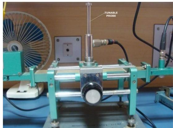
slot made in the center of the broad face do not radiate for any power of dominant mode. The precision built probe carriage having centimeters scale with a vernier reading of 0.1 mm least count is used to note the position of the probe. Additionally slotted section can be used to measure reflection coefficient and the return loss.
