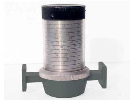
changing the cavity length. DRF measures the frequency directly. It is particularly useful when measuring frequency differences of small changes. The cylindrical cavity forms a resonator that produces a suck-out in the frequency response of the unit. This you would turn the knob until a dip in the response is observed.
